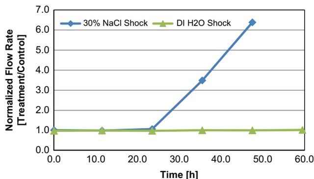
Fig. 3. The normalized flow rate through 30% NaCl and DI H<sub>2</sub>O treated membranes, respectively. The normalized flow rate was 6.5 times higher in the membrane treated with 30% NaCl than that treated with DI H<sub>2</sub>O.
