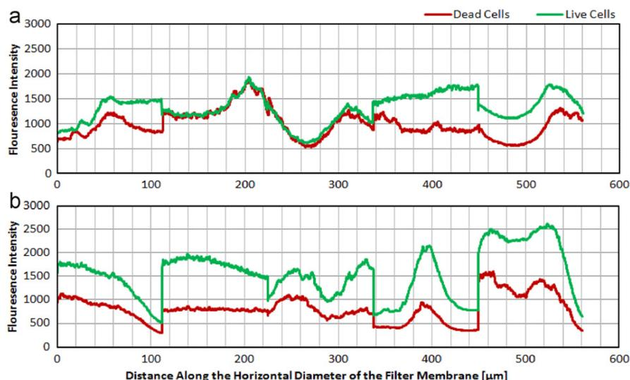
**Fig. 6.** The fluorescence profiles of the live and dead cells for the (a) 30% NaCl treated and (b) control filter membranes at 36 h using Image J. The profile was calculated by taking the average fluorescence intensity of the live and dead cells along the horizontal diameter of the filter membrane.
