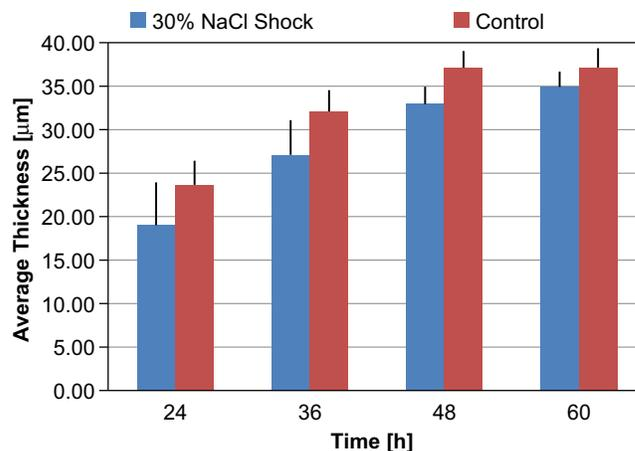
Fig. 4. The average B2 biofilm thickness (μm) on the 30% NaCl treated and control filter membranes determined using CLSM.
