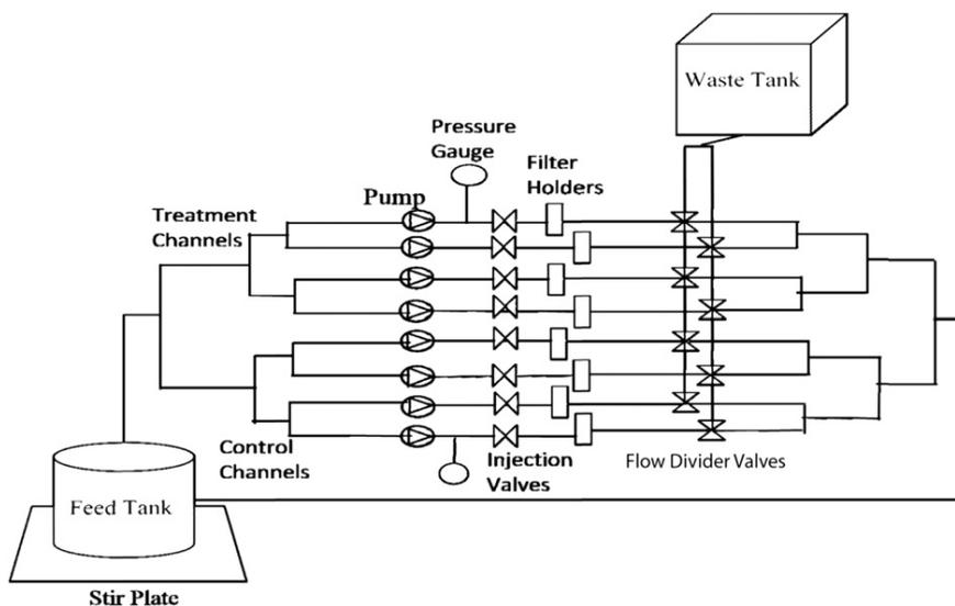
Fig. 1. Schematic of biofouling detector system.
