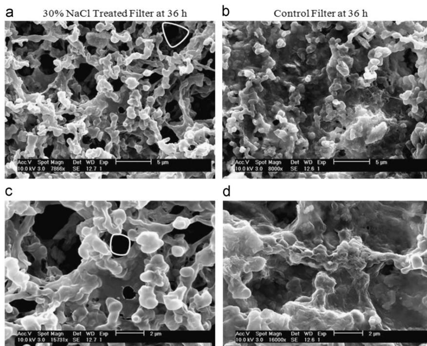
**Fig. 7.** SEM images show the biofilm morphology at 36 h during the experimental study for the 30% treated filter (a) (c), and the control filter (b) (d). The scale bars indicate 5  $\mu\text{m}$  in image (a) and (b); 2  $\mu\text{m}$  in image (c) and (d). The 'holes' between the EPS and the bacteria on the 30% NaCl treated filter membranes are depicted in (a) and (c) by the open white circles.
